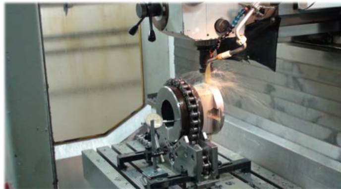
Toe-clamped directly to the machine element for reduced height
